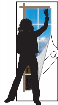
5. Roll off backing and hand-smooth mural to surface.
